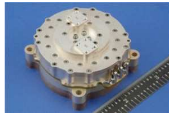
5-Watt 94 GHz Power Amplifier Module Used in SSPA
