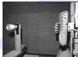
Near Field Antenna Test Range
