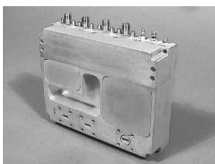
77 GHz Automobile Radar Front End
