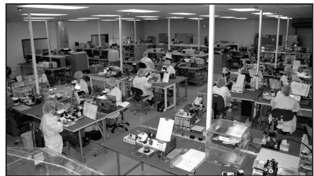
Class 10,000 Clean Room for MIC Amplifier Manufacturing
