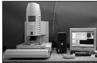
3 Axis Optical Measurement System
