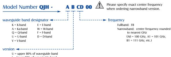
L = lower 80% of waveguide band
