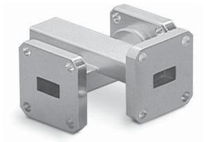
without affecting the transmitting signal. Typical applications include frequency monitoring, power sampling and built-in testing. The crossguide type of directional coupler has the advantage of lower insertion loss, smaller size and lower cost when compared to broadwall directional couplers.
